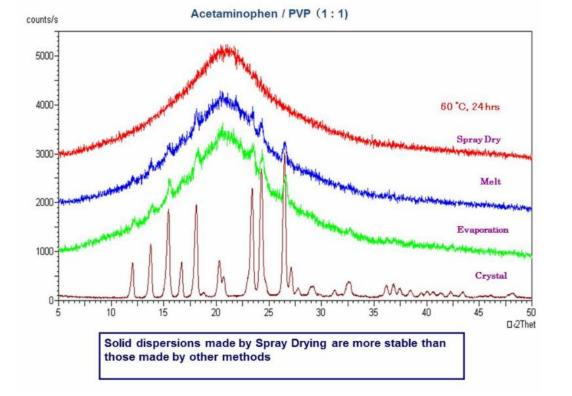
The XRD data above shows comparison study results of various solid dispersion methods using PVP as the polymer to spray dry acetaminophen, subsequently stored for 24 hours at 60 C before the analysis. The solid dispersion prepared by spray dry method indicated halo pattern in contrast with solid dispersions prepared by melt method and evaporation method, which indicated slight crystalline peaks. The study demonstrates that spray drying is more stable than other methods.
